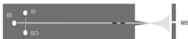
Figure 1. Schematic drawing of the microfluidic glass chip with the integrated nanospray emitter. SO: sample outlet, SI: sample inlet, BI: buffer inlet, MS: mass spectrometer.
